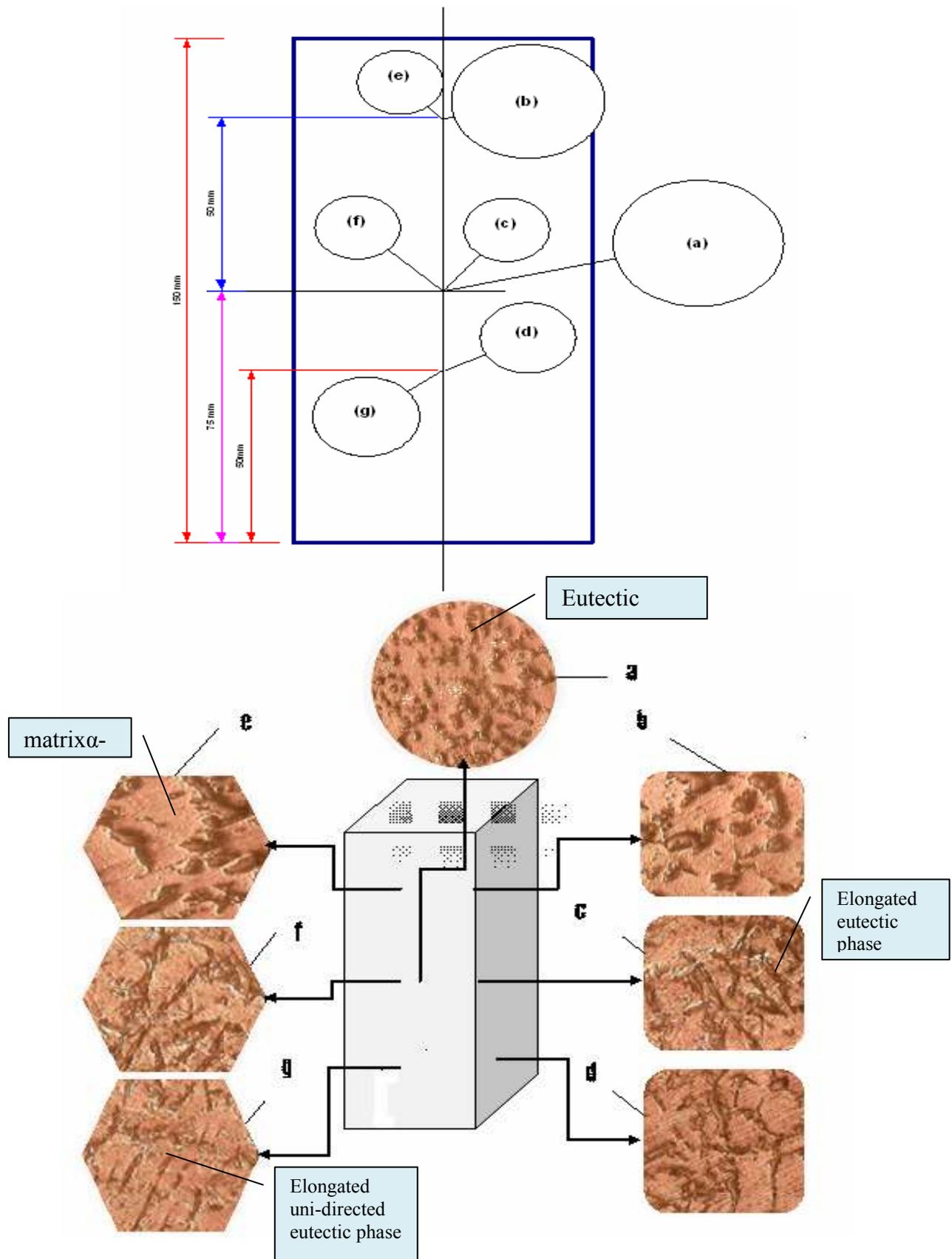
Figure (3): A schematic diagram of the resulted microstructure for
