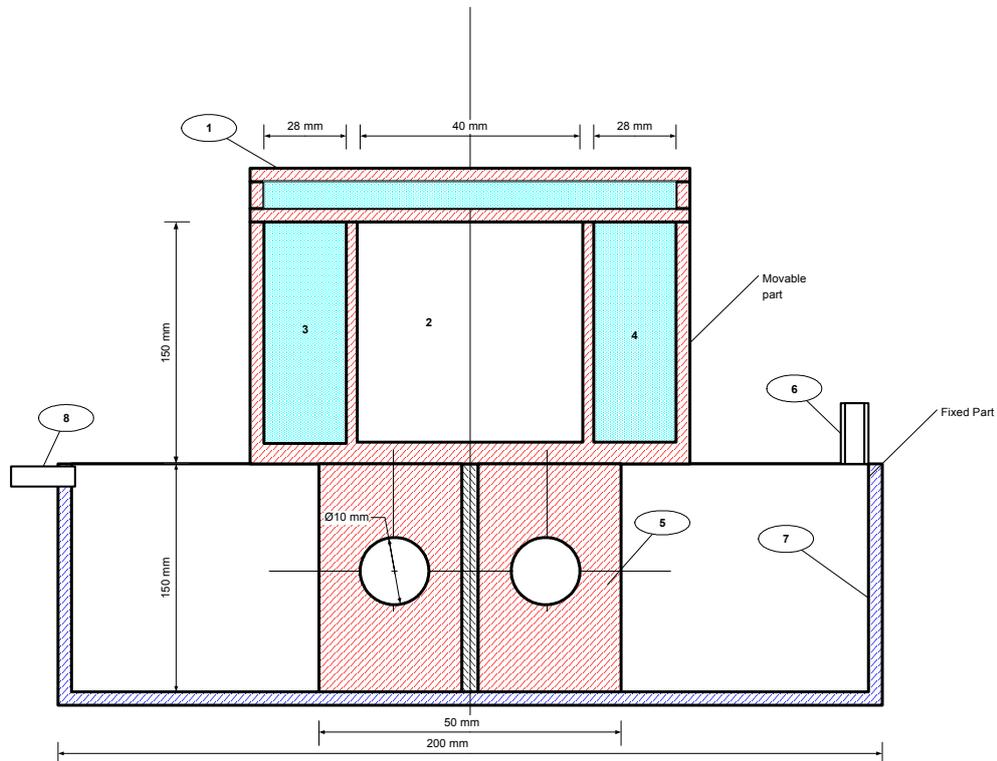
1. Insulated cover, 2. Mold cavity, 3 & 4. Cavity for insulation, 5. Double fin, 6. Cold water inlet, 7. Reservoir (lower part), 8. Water outlet.
