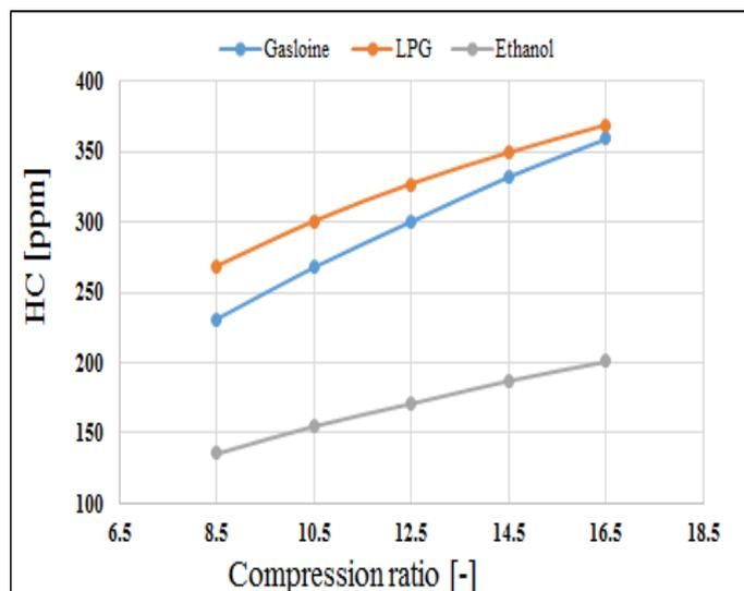
Fig.7. Variation of HC\_Gasoline\_LPG\_Ethanol at 2500 rpm vs. compression ratio
