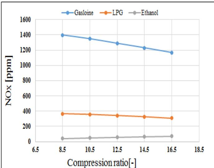
Fig.8. Variation of NO<sub>x</sub>\_ Gasoline\_ LPG\_ Ethanol at 2500 rpm vs. compression ratio
