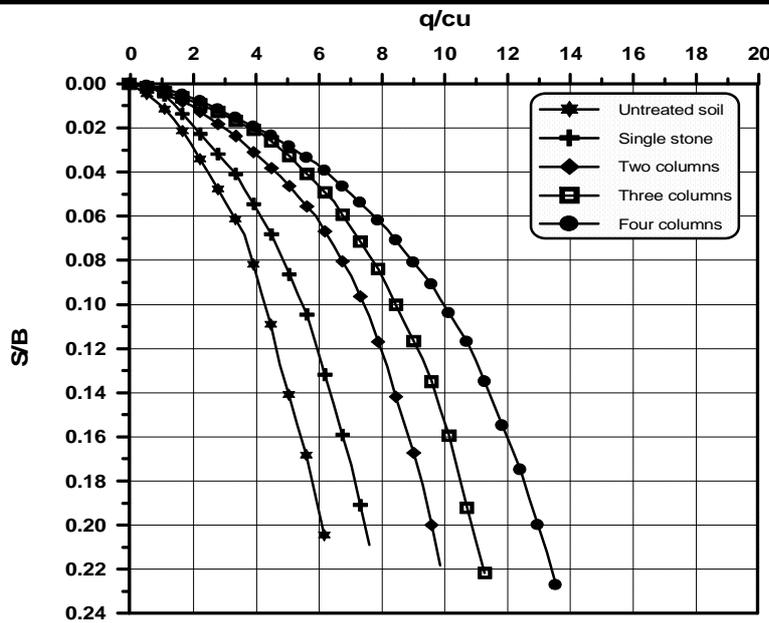
Figure (13)  $q/c_u$  versus  $S/B$  for soil treated with stone column
