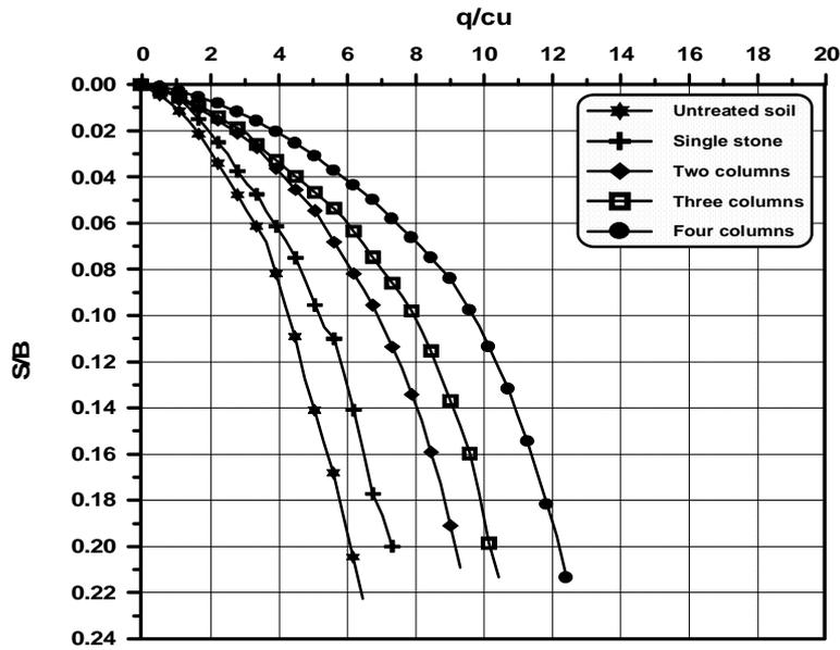
Figure (7)  $q/c_u$  versus  $S/B$  for the soil treated with stone column,  $c_u = 6$  kPa and  $L/D = 6$ .
