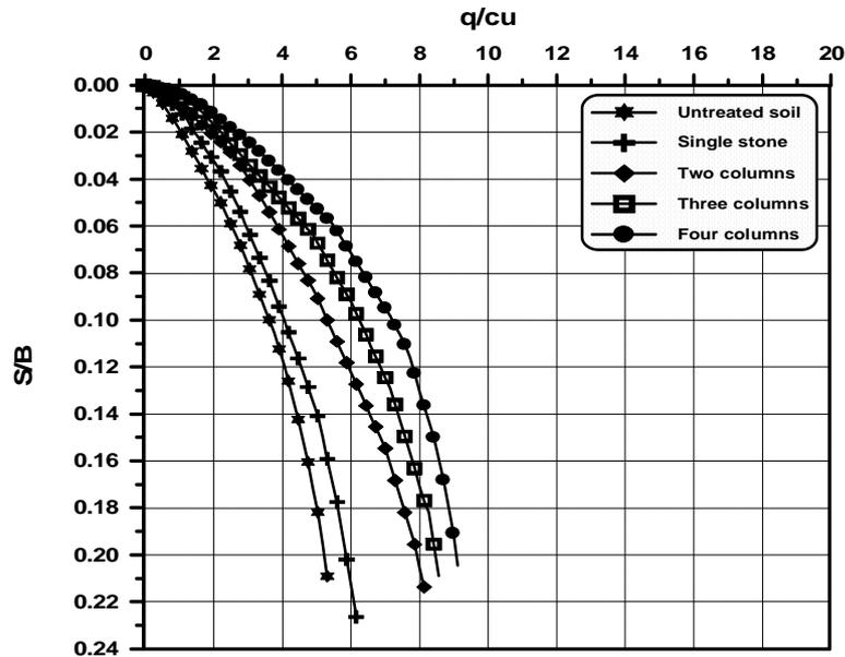
Figure (17)  $q/c_u$  versus  $S/B$  for the soil treated with stone column  $c_u = 12$  kPa and  $L/D = 8$ .
