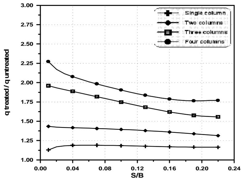
Figure (10) Bearing improvement ratio versus ( $S/B$ ) for the soil treated with stone columns,  $c_u = 9$  kPa and  $L/D = 6$ .
