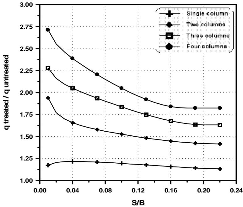
Figure (16) Bearing improvement ratio versus ( $S/B$ ) for the soil treated with stone columns,  $c_u = 9$  kPa and  $L/D = 8$ .
