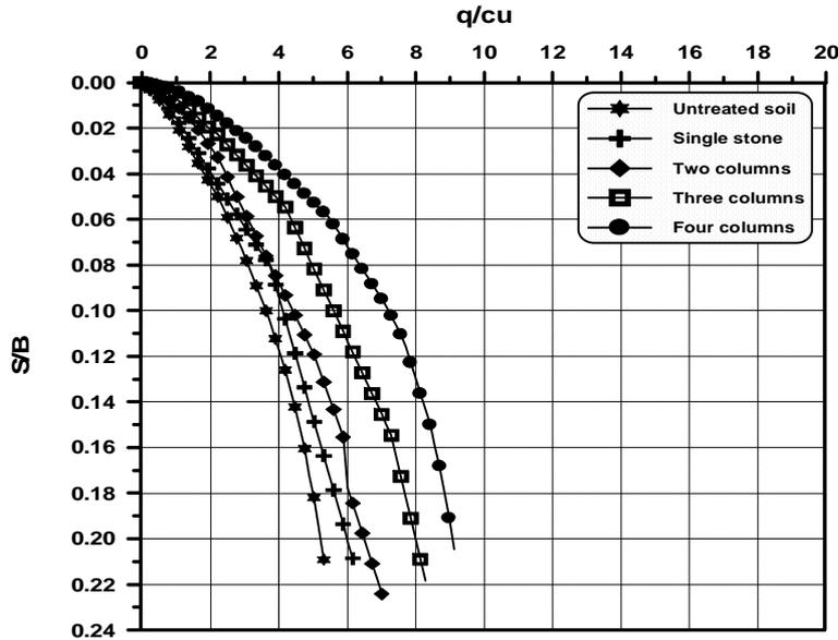
Figure (11)  $q/c_u$  versus  $S/B$  for the soil treated with stone column,  $c_u = 12$  kPa and  $L/D = 6$ .
