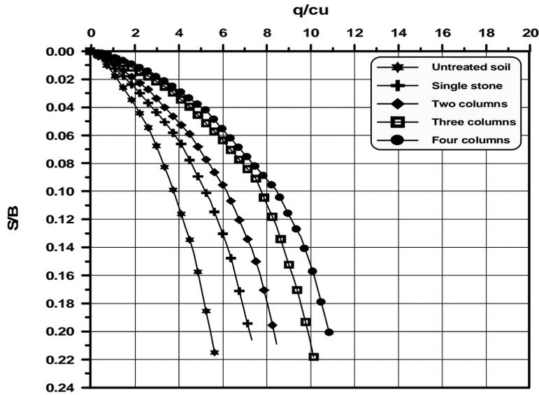
Figure (9)  $q/c_u$  versus  $S/B$  for the soil treated with stone column,  $c_u = 9$  kPa and  $L/D = 6$ .
