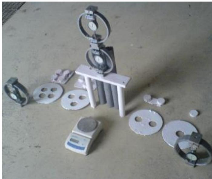
Figure (3) Foundation plates and accessories.
