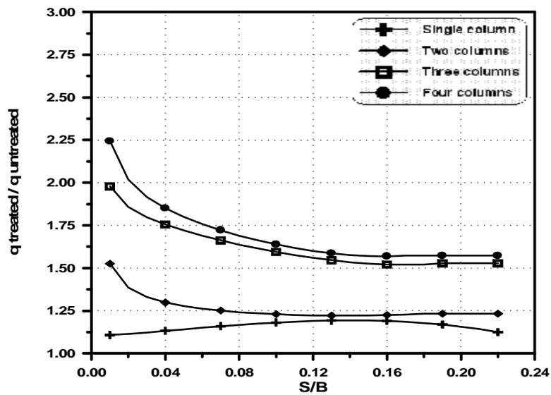
Figure (12) Bearing improvement ratio versus  $(S/B)$  for the soil treated with stone columns,  $c_u = 12$  kPa and  $L/D = 6$ .
