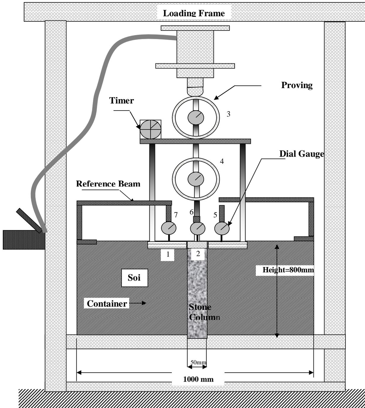
Figure (4) Schematic diagram of the experimental set-up.
