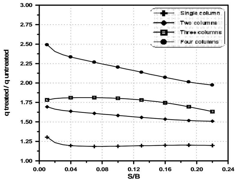
Figure (8) Bearing improvement ratio versus ( $S/B$ ) for the soil treated with stone columns,  $c_u = 6$  kPa and  $L/D = 6$ .
