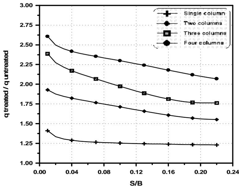
Figure (14) Bearing improvement ratio versus  $(S/B)$  for the soil
