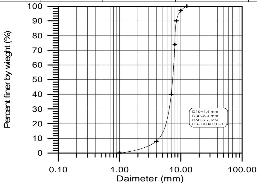
Figure (1) Grain size distribution of the crushed stone used in preparing the model tests.
