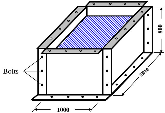
Figure (2) Steel container used in the tests.
