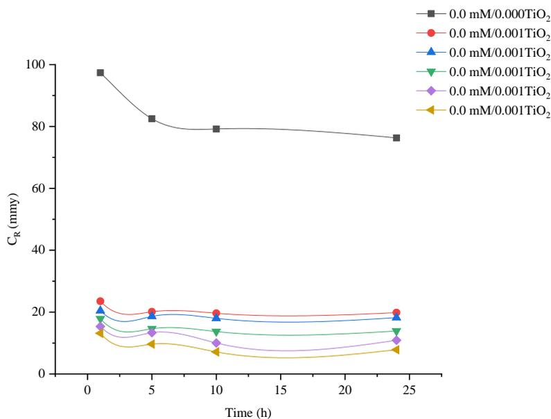
**Figure 6.** Influence of concentration of BPTA synergistic with 0.001 g, of TiO<sub>2</sub>-NP in 1 M HCl and time on the corrosion rate of MS.
