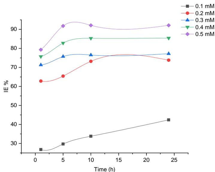
**Figure 1.** Immersion time impact of MS in a corrosive environment at various concentrations of BPTA.
