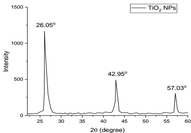
**Figure 12:** The X-ray characterization of  $\text{TiO}_2$ -NP.
