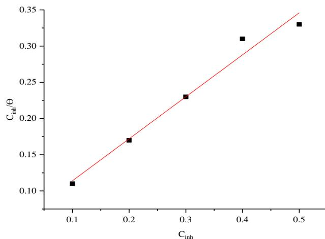
**Figure 8.** Langmuir plot for adsorption of corrosion inhibitor molecules of BPTA synergistic with 0.001 g of  $TiO_2$ -NP on to MS.
