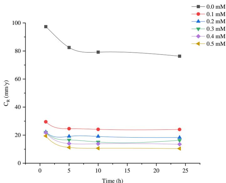
**Figure 5.** Impact of BPTA concentration and corrosion rate of MS with immersion time
