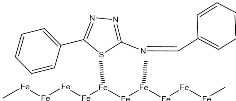
**Figure 10.** Suggested mechanism of action of the BPTA.
