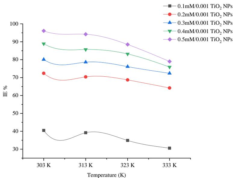
**Figure 4.** Temperature impact on inhibition efficiencies of BPTA synergistic with 0.001 g, of TiO<sub>2</sub>-NP in 1 M HCl.
