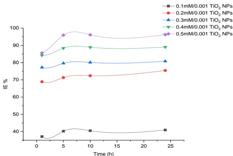
**Figure 2.** Immersion time impact of MS in a corrosive environment at various concentrations of BPTA synergistic with 0.001 g, of TiO<sub>2</sub>-NPs.
