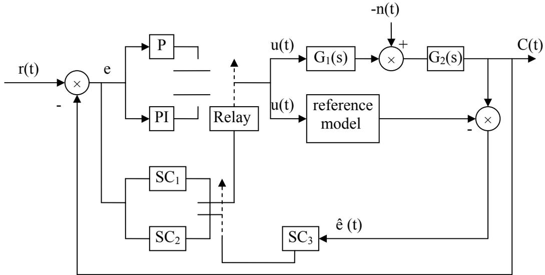
Fig (9) adaptive VSS using (P&PI) controller
