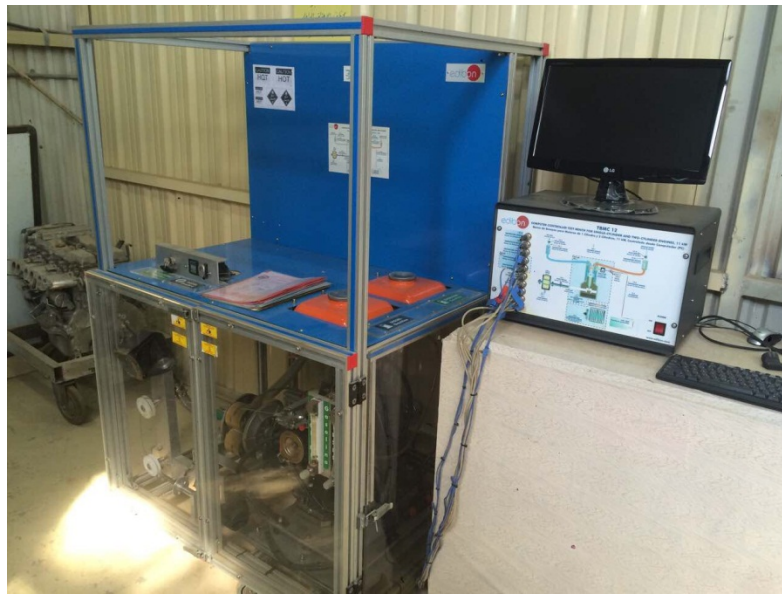
Fig. 1: Photograph of the rig including the engine and the computer-controlled unit.
