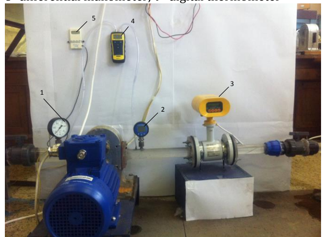
Fig -4: Measuring instruments from the experimental installation 1- Bourdon manometer; 2- Barolli manometer; 3- electromagnetic flow meter; 4- differential manometer; 5- digital thermometer
