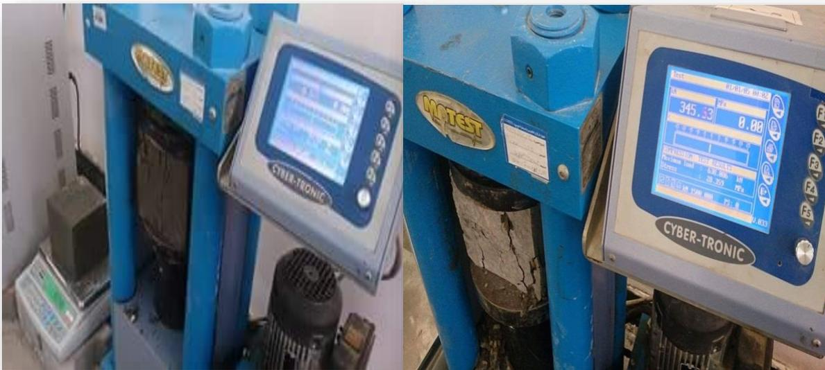
Figure.4 : Cube samples during compression test
