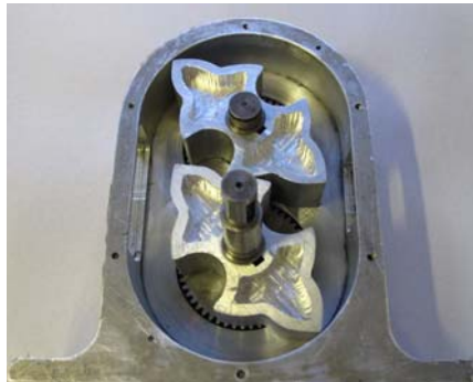
Fig.6. Specially profiled rotor mounted in the case
