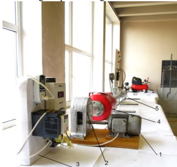
Fig.10. Overview of the experimental installation 1 electric motor; 2 - rotating blower; 3-panel with electrical appliances; 4- compressed air tank; 5-diaphragm for air flow measurement
