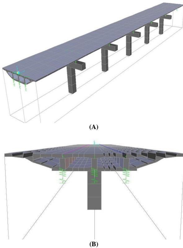
Fig. 2: Continuous Box Girder Concrete Bridge Model: (A) Longitudinal Section, (B) Transverse Section.
