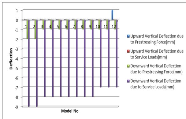
Fig. 6: Vertical Deflection Values of Continuous Box Girder Bridge Model.
