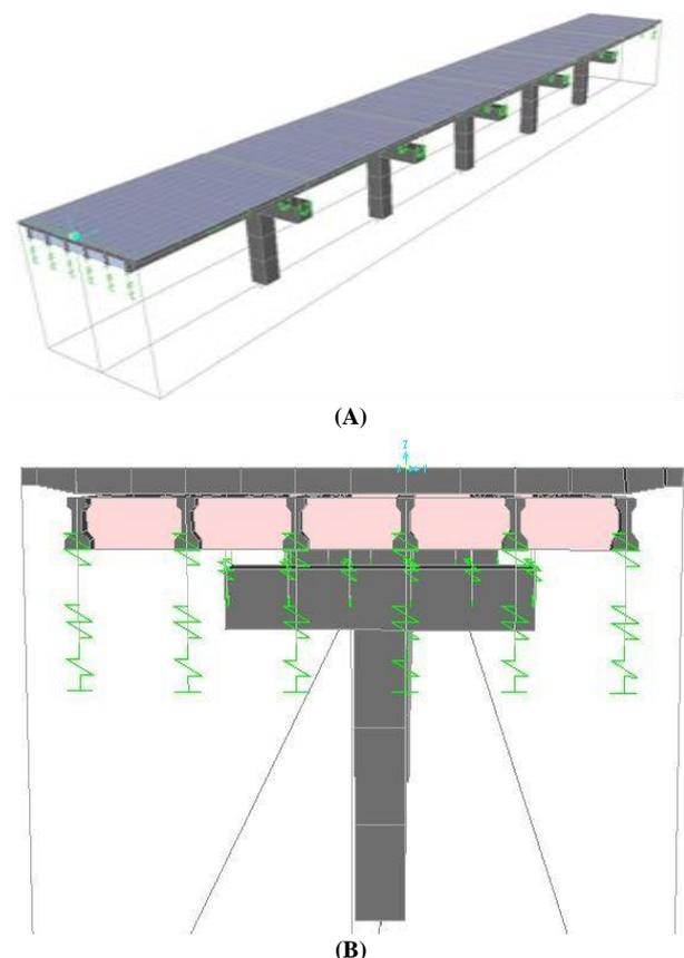
Fig. 1: Simply-Supported I Girder Bridge Model: (A) Longitudinal Section, (B) Transverse Section.
