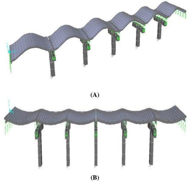
Fig. 3: Vertical Deflection of Simply-Supported I-Girder Prestressed Concrete Bridge Model: (A) Due to Prestressing Tension Force, (B) Due to Service Loads.
