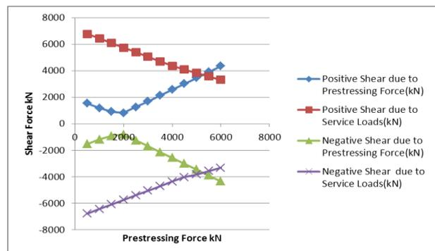
Fig. 8: Vertical Shear Force of Continuous Box Girder Bridge Model.
