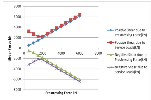
Fig. 7: Vertical Shear Force of Simply-Supported Bridge Model.
