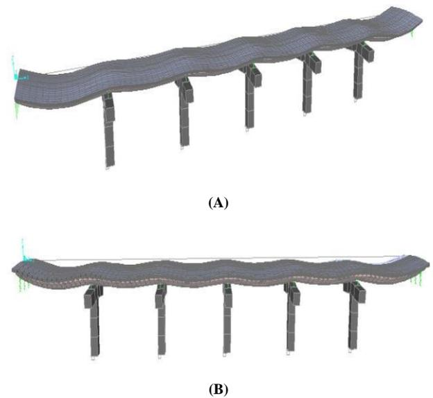
Fig. 4: Vertical Deflection of Continuous Box Girder Prestressed Concrete Bridge Model: (A) Due to Prestressing Tension Force, (B) Due to Service Loads.
