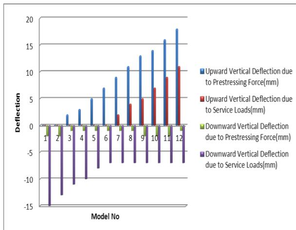
Fig. 5: Vertical Deflection Values of Simply-Supported Bridge Model.
