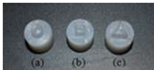
Figure 2. Types of indenters employed:(a) circle; (b) square; (c) triangle.
