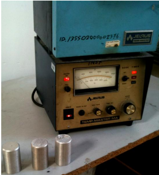
Fig. 8. Homogenizing Aluminum Billet in a Furnace.
