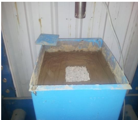
(c): Partial replacement (square footing)
