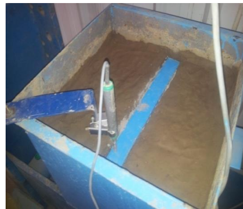
(d): Strip footing during the test
