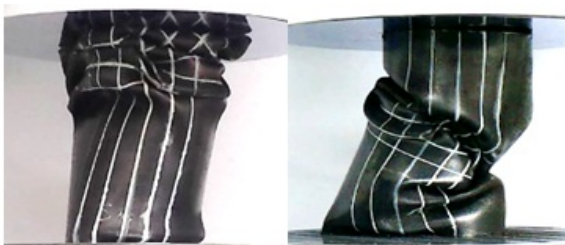
Figure-12. Deformation of the tube with holes in the middle (a) before irregular deformation (b) after irregular deformation.
