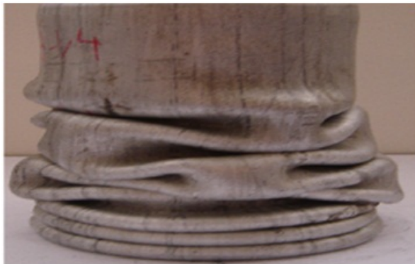
Figure-7. Mix-mode deformation the fold started to ring and transfer to lobes [19].
