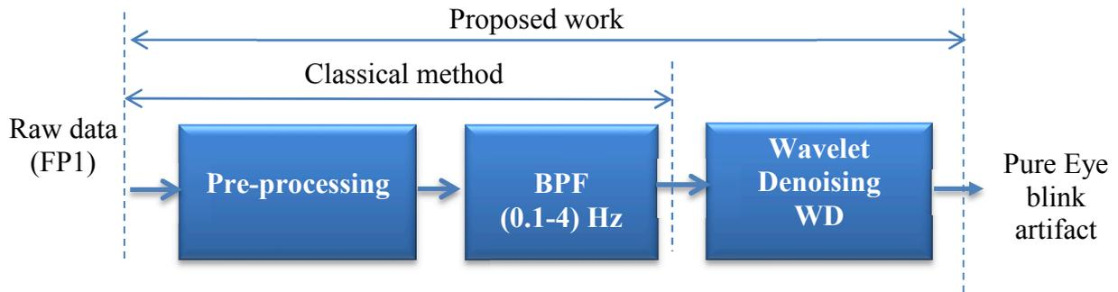
FIGURE 3. Block diagram of the proposed approach: Enhanced Channel-Reference algorithm
