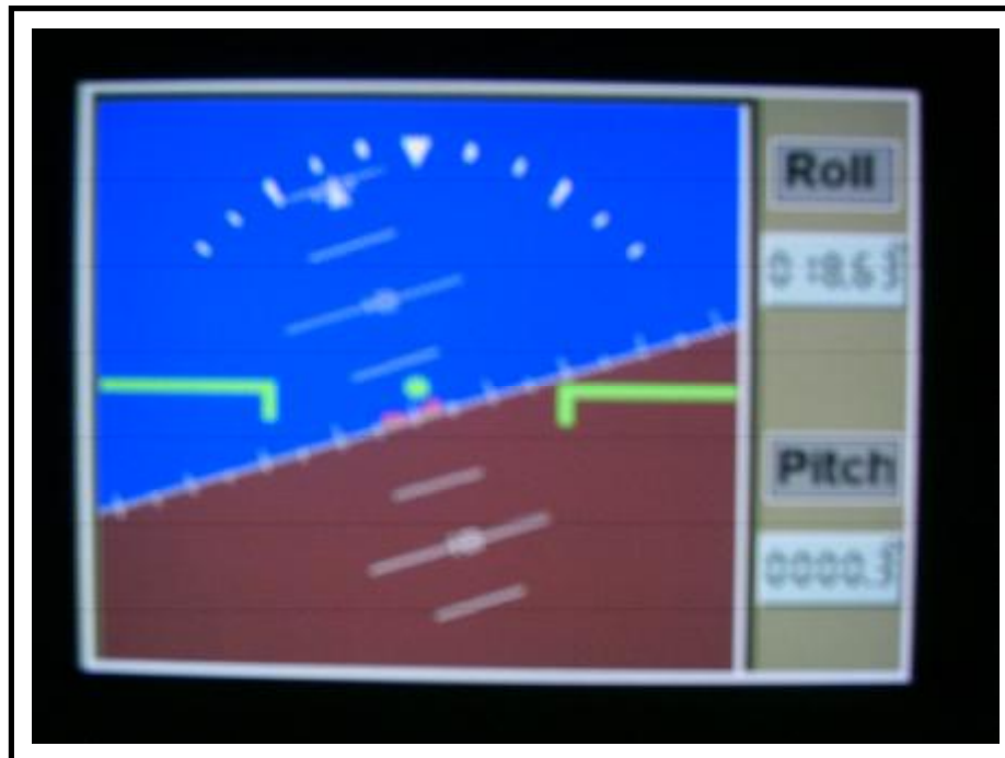
Fig.(4) Roll and Pitch Angles Measurements at 18.63 and 0.3 degrees Respectively.
