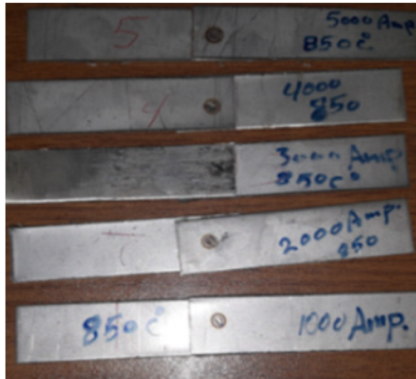
Figure 2. Annealing temperatures for weldments
