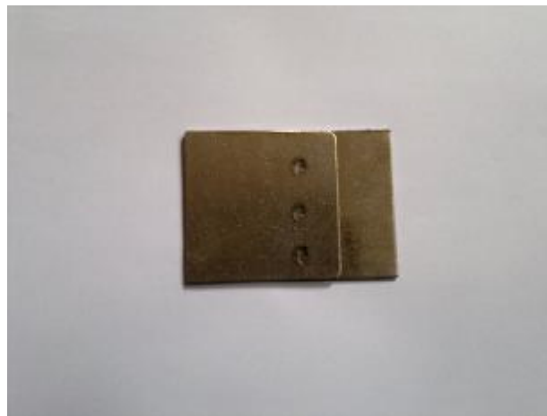
Figure (2): Plate after heat treatment, spot welding and shot peening.
