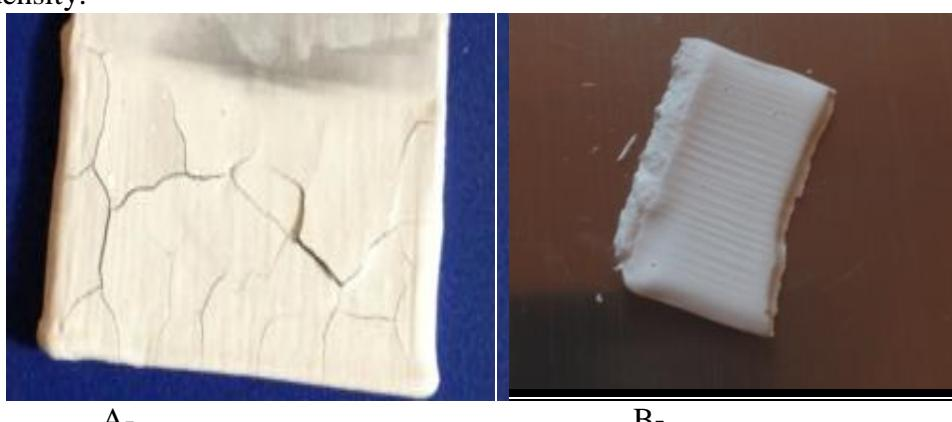
**Figure (1): Effect the type of DC voltage; A- constant voltage (250V), B- Variable voltages (250-290 V).**
