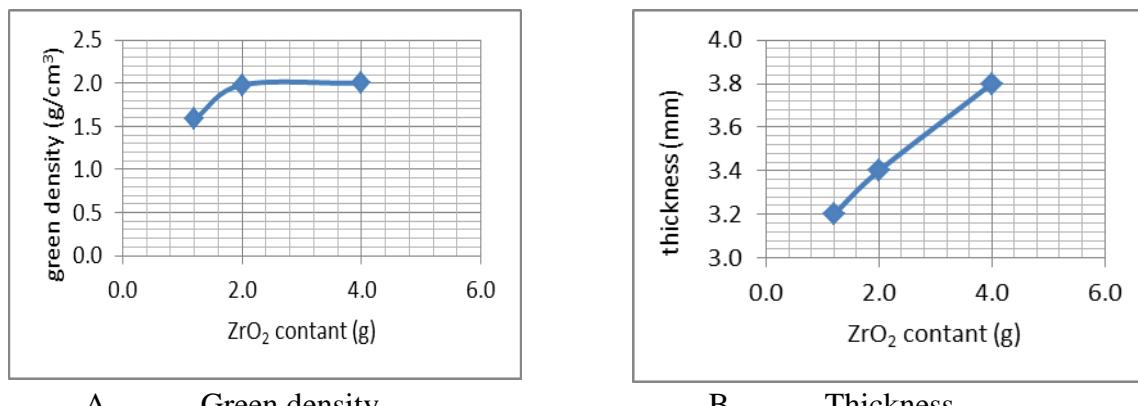
**Fig(3): effect of ZrO<sub>2</sub> on green density and thickness of deposited zirconia from 1g PEG in 100 ml ethanol suspension. A- Green density, B- Thickness.**
