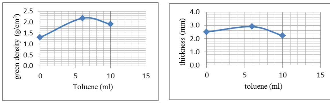
**Fig(7): effect of toluene on thickness and green density of deposited zirconia from 1.2g zirconia in 1.5g PEG -100 ml ethanol suspension. A- Green density, B- Thickness.**
