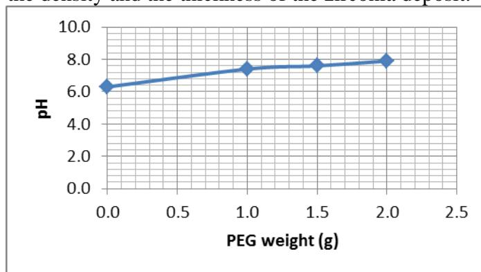
**Fig(4): effect of PEG on pH of 4g zirconia in 100 ml ethanol suspension.**
