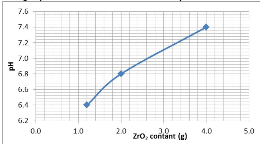
**Fig(2): effect of ZrO<sub>2</sub> on pH of 1g PEG in 100 ml ethanol suspension.**
